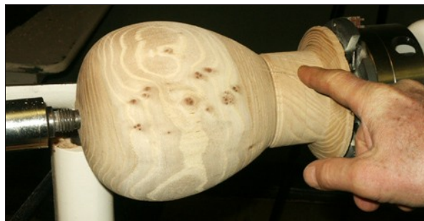
Vessel Foot Preparation
