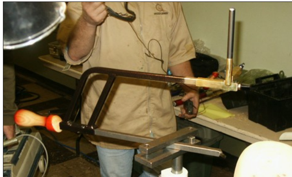
Above Don's Hollowing Tool - Below Tool at work
