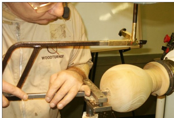
Above Don's Hollowing Tool - Below Tool at work
